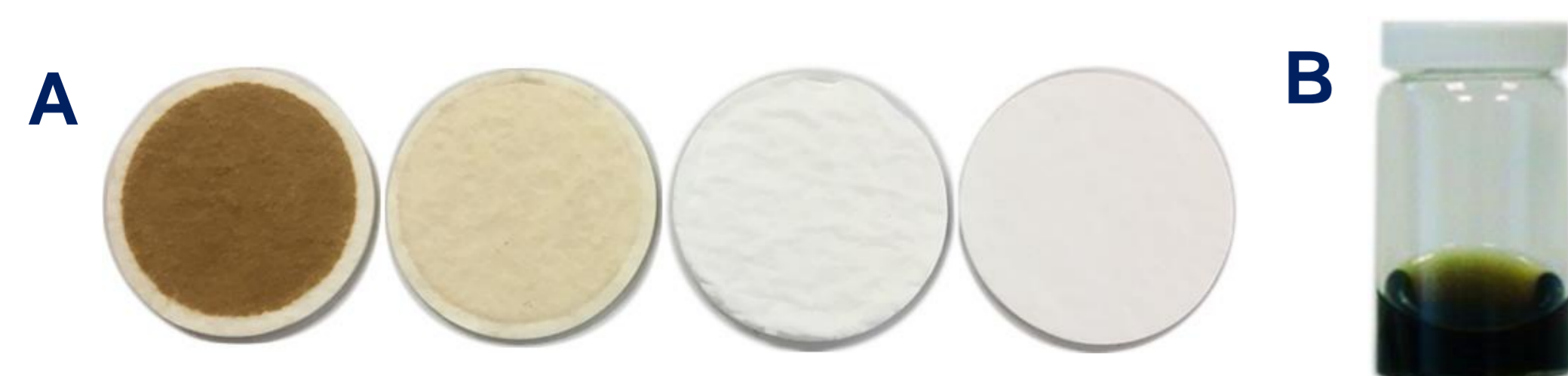
Figure 2: A) Representative CFP from 3R4F (10 puffs), Glo™ (48 puffs), e-cig (500 puffs) and blank. B) 3R4F PM eluted in DMSO.
